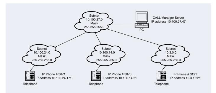
Figure 2: Network Subnet Configuration for IP Phone Evaluation
