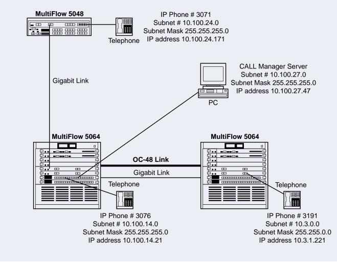
Figure 4: Configuration for Fault Tolerance Evaluation by AQR
