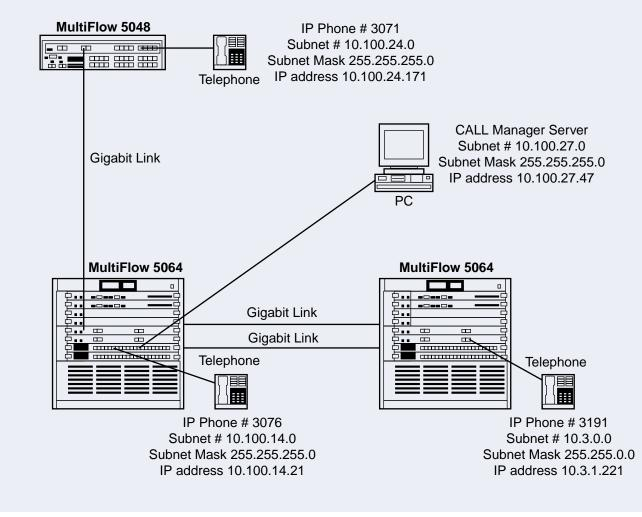
Figure 5: Configuration for Fault Tolerance Evaluation by Link Aggregation
