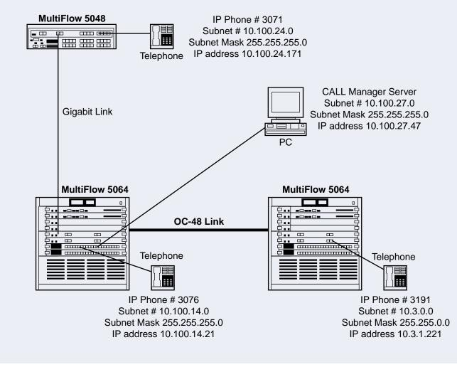
Figure 3: Network Physical Configuration for IP Phone Evaluation
